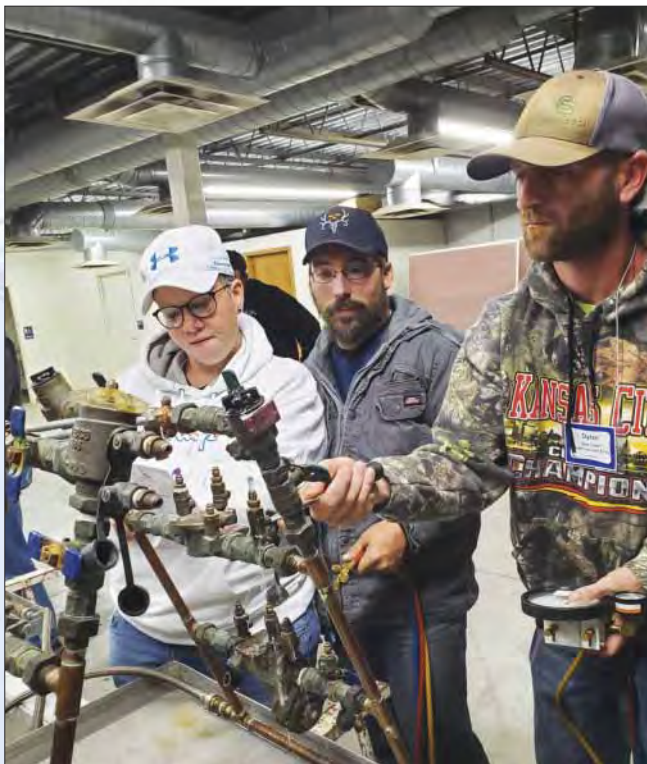
Dylan Tolbert with GreenTouch Lawn & Tree and apprentices Kylee Nikkle and Jeff Stigge from the city of Washington practice testing backflow preventers during KRWA-sponsored training at Grandview Plaza in December 2022.
